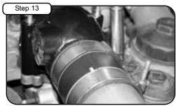
Tighten the clamp using 7/16" socket. See notes 2 & 4
