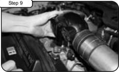
Carefully guide manifold into coupler hose.
