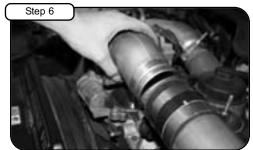
Remove stock manifold out of vehicle.
