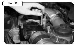
Apply threadlocker to all screws. Secure manifold with flat washers and screws.
