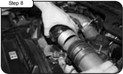
Install 1/8" NPT plugs to back of manifold. Tighten using 3/16" allen key. Install new aFe BladeRunner manifold to vehicle. See notes 2 & 3.
