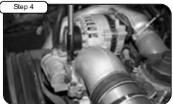
With 10mm socket and extension, loosen the 1 screw closest to passenger headlight.
