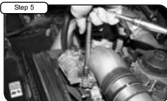
With 8mm socket and extension, loosen the 3 remaining
