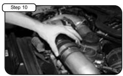
Slide back clamp. Do not tighten.
